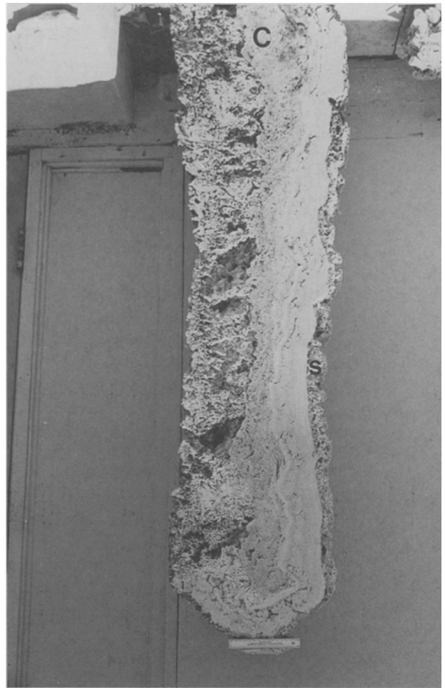
Figure 4. Longitudinal section of the studied stalactite (oriented in original growth position) showing its internal structure. The porous half was buried in unlithified sediment as it rested horizontally on the ledge from which it was retrieved. Ruler is 6 inches long. "C" is the calcite core; "s" is the skeletal rind.
